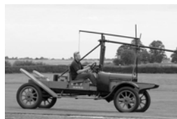
'Hucks' engine starter for spinning up the props
